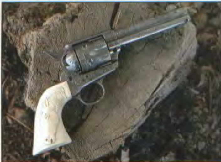
A 1 st Generation Colt SAA engraved with Helfricht style "C" coverage by the late Charles Baker. The shot-out barrel and cylinder was replaced with custom 2 nd Generation parts. The cylinder was beveled and refluted and rechambered with tight .452 throats. A cut and crowned 7-1/2" barrel was installed with the proper front sight. Period correct caliber markings and address were applied along with an 11-degree forcing cone. It was plated with antique silver plating and fire blue screws and elephant ivory one piece grips with a carved horse head were added. Finally, it was given a "Gunslinger" action job with a 2.5 lb. trigger pull.
