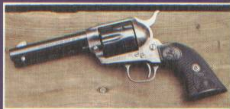
Eddie Janis tuned up this Colt Model P .38 WCF with his custom Gunslinger action package – including a 3-pound trigger pull.
